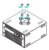
Attach the other VESA Bracket to the rear of a compatible display using the four screws.
